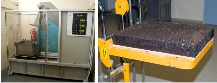
Figure 5.3: Rolling compactor WSV-2008-KW50/500 and the resulting 500 mm 2 slab
